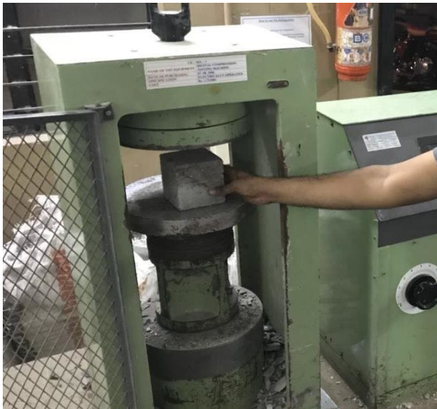
Fig. 3 A view of UCS test and schematic diagram of device (updated from Reinhardt, 1991)
